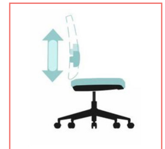
Lumbar support height adjustment
